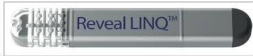
Figure 2: Reveal LINQ insertable cardiac monitor.
